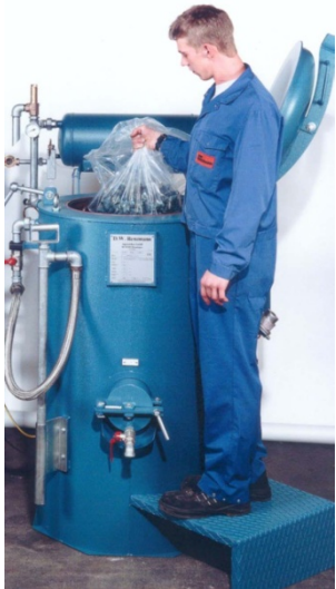
Sludge Removal with Nylon Bag or via clea-out-hatch
